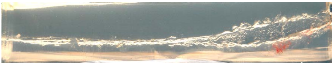
Fig. 2 Transmitted light print of a 25-cm-long bullet track of series 1. Near the bullet exit, red textile fibres transferred in a retrograde direction are macroscopically visible
